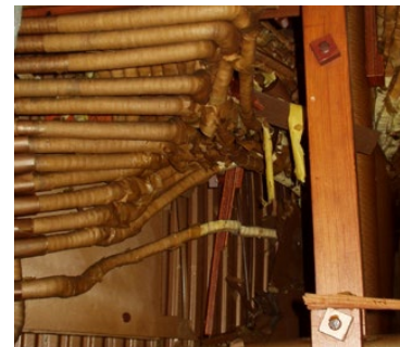
Displaced internal connections
